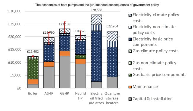
Figure 6: Net present cost of heating systems
