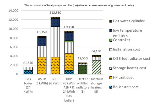
Figure 4: Upfront costs of heating systems for a typical semi-detached UK household (central cost
