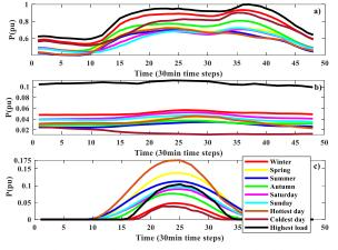
Figure 1. Active power of representative profiles for a) load, b) wind and c) PV generation.
