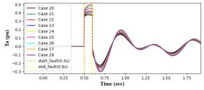
Figure 5. Accelerating Torque for SG3 for Cases 20-28. Fault on line 4-5.
