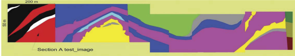
Figure 3. Geotechnical section A, with total length of 1.2 km. The arrow shows the “TEST- Ground Truth” image for this section.
