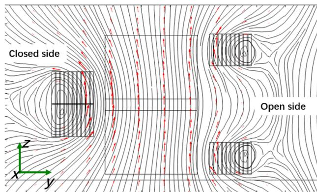
FIG. 7. Distribution of magnetic flux generated by HTS-stacked ring magnet.
