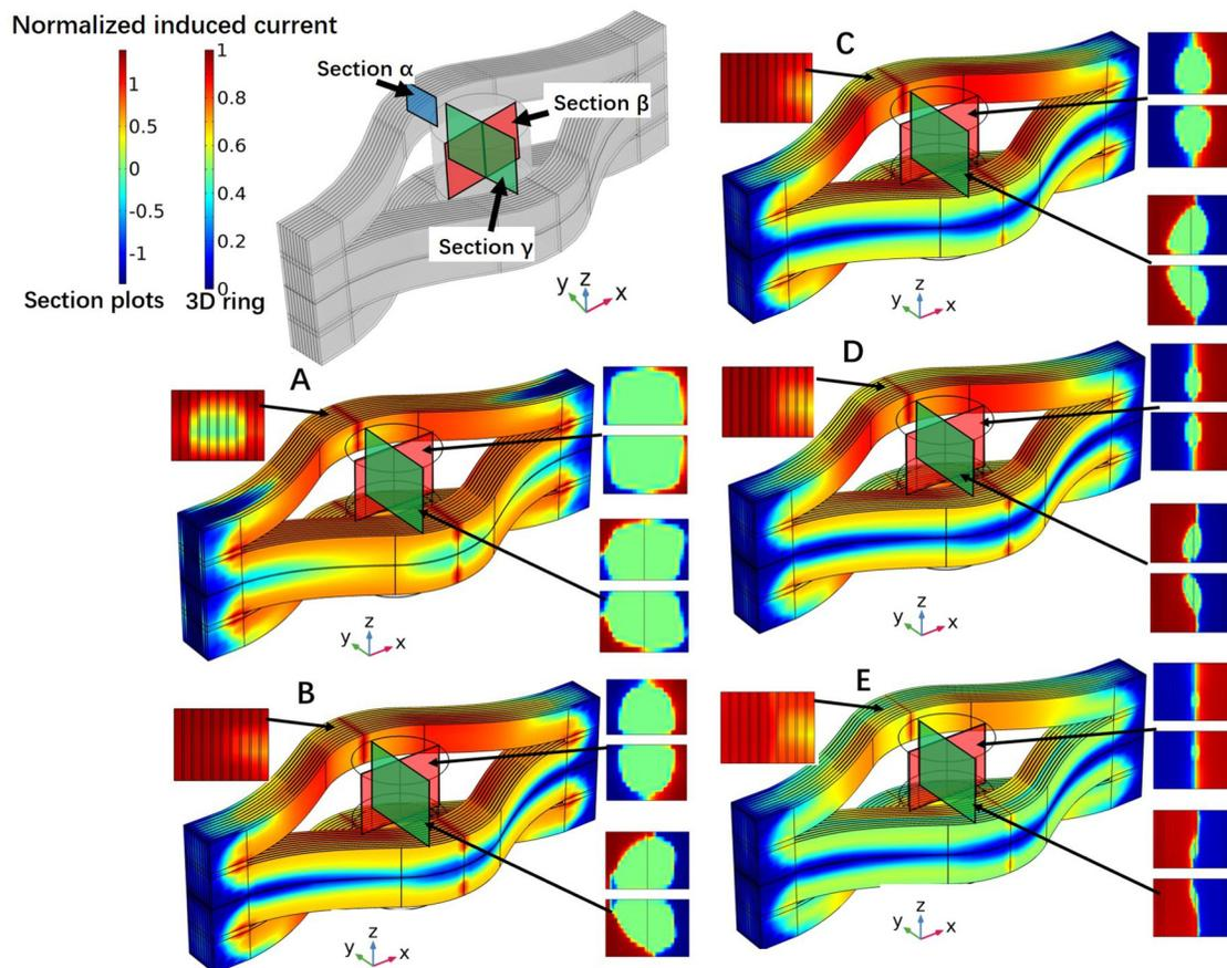
FIG. 6. Plots of the spacial current distribution profiles when the applied field is ramped down to 6 (a), 4 (b), 2 (c), 0 T (d), and after flux creep (e).
