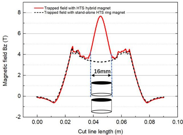
FIG. 3. Trapped field distribution along the center cut line of the HTS hybrid magnet and stand-alone HTS-stacked ring magnet.
