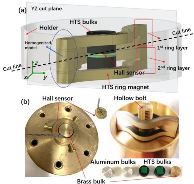
FIG. 1. The HTS hybrid trapped field magnet design: (a) scheme of the hybrid magnet design; (b) physical picture of the design. The measurements were carried out with two HTS bulks or two aluminum bulks for comparison.
