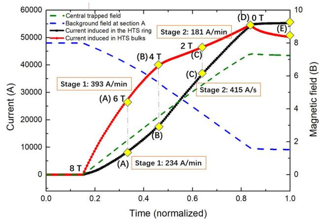
FIG. 5. Current increase in the cross sections of the HTS hybrid magnet.
