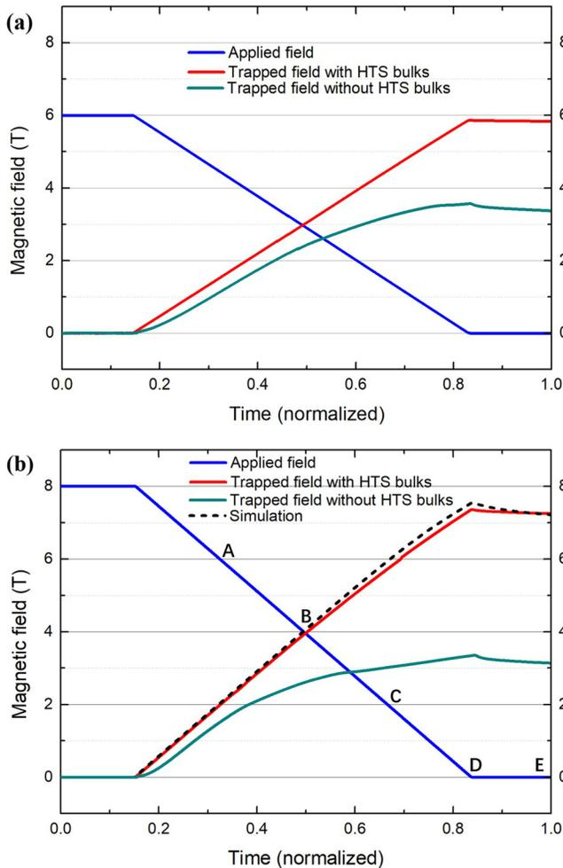
FIG. 2. Field cooling magnetization results at 25 K with a 6 T applied field (a) and an 8 T applied field (b).
