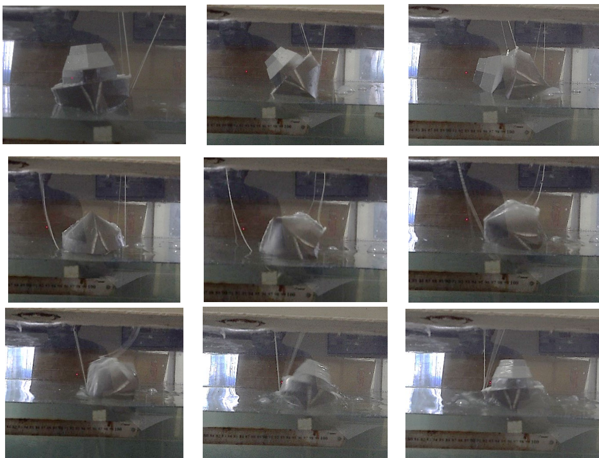
Figure 11. Physical model for self-righting moment at 180°.
