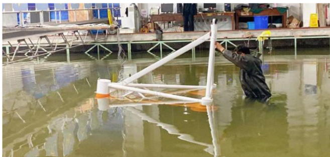
Fig. 16. Free decay test in the physical tank.
