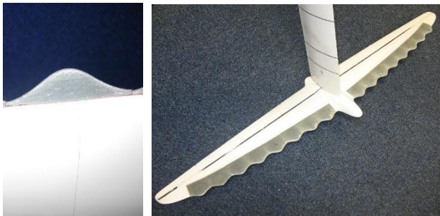
Figure 8 - Foil with Full Coverage of Tubercles
