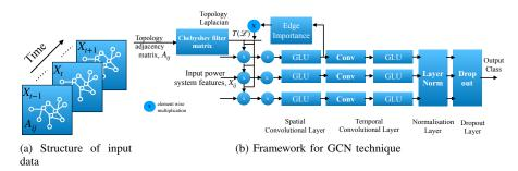
Fig. 1: Spatio-temporal GCN framework for predicting cascading failure
