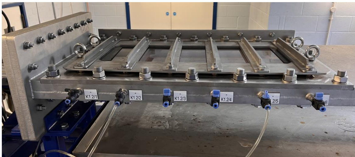
Figure 4. Pressure taps distribution numbered from 1 to 6 (left to right) on the test section of the FTFC.
