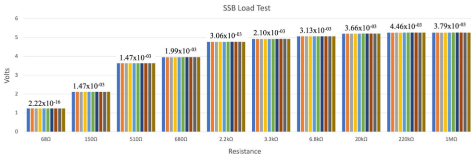
Figure 3. Resistance & Load Testing Results with Standard Deviation Values
