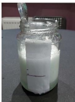
The impact of temperature on a reaction is even more evident if a small amount of washing up liquid is added to capture the gas produced. The foam produced lasts longer than the gas bubbles alone would, which aids measurement.
