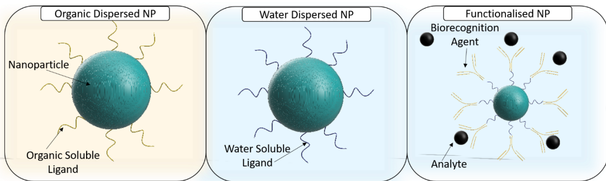
Figure 7: Nanoparticles with different ligands imbuing them with different properties, from left to right: organic ligands on NPs in organic media, aqueous ligands on NPs in aqueous media and aqueous ligands on NPs attached to biorecognition agents selectively binding to analytes in aqueous media
