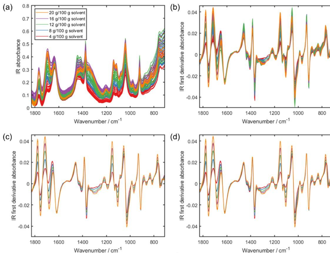
**Figure 2.** Overlay of IR calibration spectra acquired for different concentrations of LAA in MeCN/H<sub>2</sub>O (80:20 w/w): (a) all absorbance spectra, (b) all first derivative spectra, (c) first derivative spectra acquired at 50 °C, and (d) first derivative spectra transformed via LSS so they are as though they were acquired at 50 °C.
