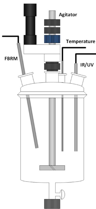
**Figure 1.** Schematic of the experimental setup. The vessel shown was used as part of the OptiMax platform including temperature, focused beam reflectance measurement (FBRM), and IR or UV probes.
