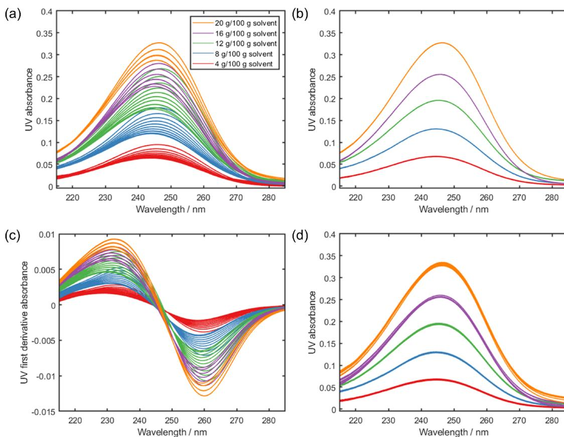
**Figure 3.** Overlay of UV calibration spectra acquired for different concentrations of LAA in MeCN/H<sub>2</sub>O (80:20 w/w): (a) all absorbance spectra, (b) absorbance spectra acquired at 50 °C, (c) all first derivative spectra, and (d) all absorbance spectra after transformation via LSS so they are as though they were acquired at 50 °C.
