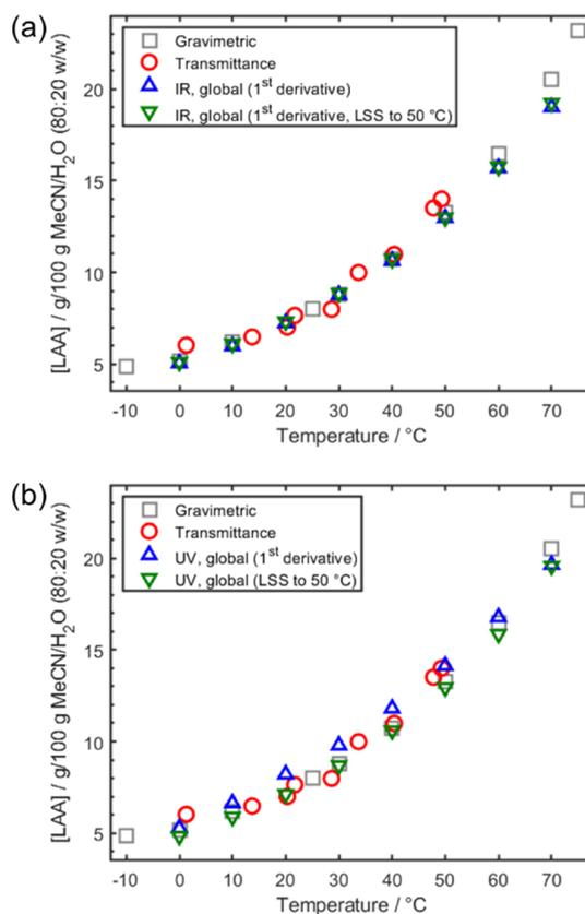
**Figure 4.** Variable temperature solubility diagrams for LAA in MeCN/H<sub>2</sub>O (80:20 w/w) obtained using gravimetric, transmittance, and (a) IR and (b) UV methods.
