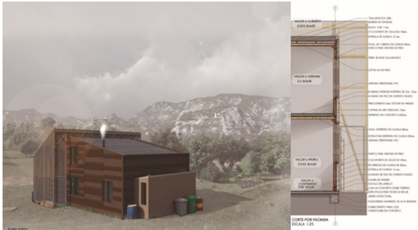
Figure 8 Image of the Colombian solution for Passivhaus using Bio Materials.
