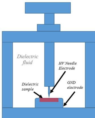
Fig. 1. Schematic of test cell used for all breakdown experiments.
