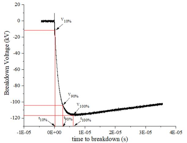
Fig. 2. Example of one of the discrete voltage wave-forms (nominal rise-time 0.4 μs) applied during breakdown tests. Nominal rise-time of the impulse was taken as the time for the magnitude to increase from  $V_{10\%}$  to  $V_{90\%}$  with a multiplication factor of 1.25 applied [14].
