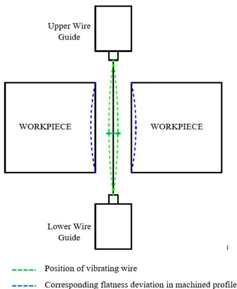
Fig. 2. Representation of geometrical inaccuracy (flatness error) caused due to wire vibrations
