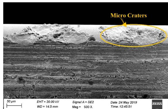
Fig. 5 a). SEM image of brass wire after machining
