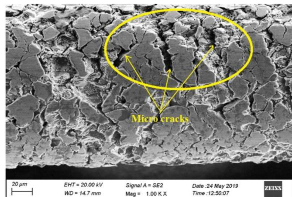
Fig. 5 b). SEM image of Zn coated brass wire after machining
