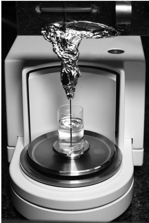
Figure 4: Gravimetric setup at DTI. Weighing scale with a glass beaker and the immersed needle in water with an oil layer on top of it.
