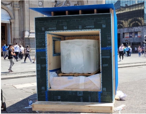
Figure 4: Passivhaus box with the ice inside at the beginning of the 10 days (before closing the box - 1000 kg of ice). Source: Authors.
