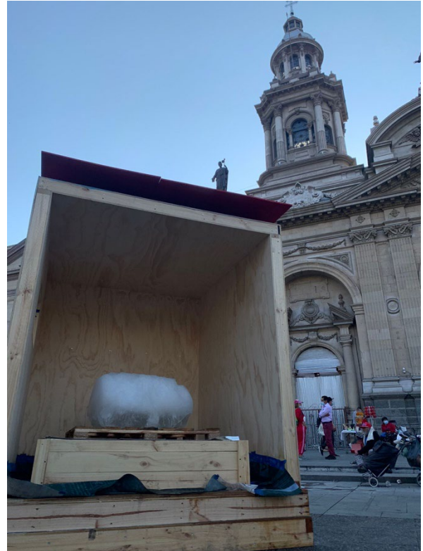
Figure 6: Local regulations box with the ice inside after 10 days (230 kg of ice). Source: Authors.
