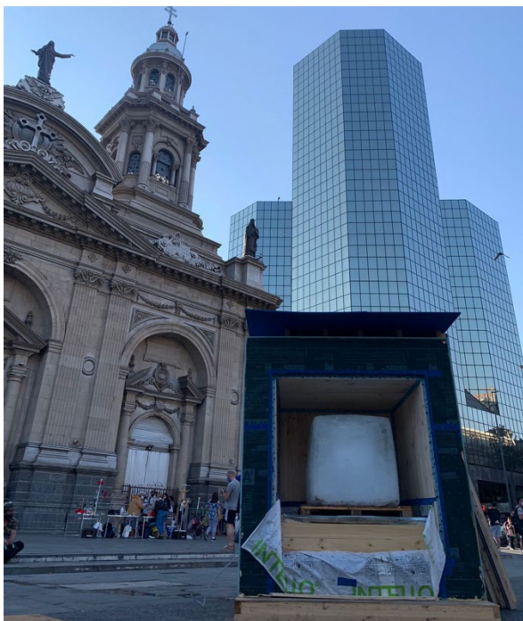
Figure 5: Passivhaus box with the ice inside after 10 days (645 kg of ice). Source: Authors.
