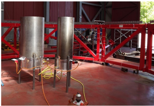
Fig. 8. Dual burner test with the ring lying horizontal.
