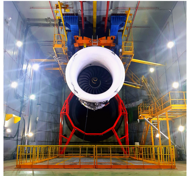
Fig. 1. Optical mounting frame (red) behind a large scale commercial aero-engine at the engine test bed facility at Instituto Nacional de Tecnica Aeroespacial (INTA), Madrid.
