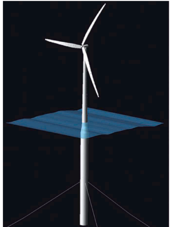
Fig. 1. Floating Offshore Wind Turbine System, adapted with permission from ( Jonkman and Matha, 2011 ).
