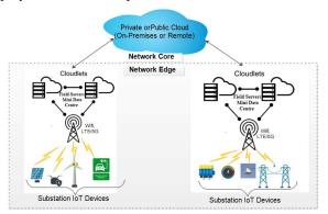
Figure 1. Proposed Cloudlets Supported Smart Grid to Reduced Substation-to-Substation Latency
