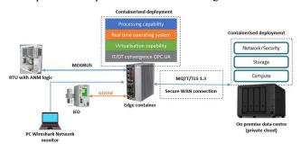
Figure 2. High-Level Cloudnet Test Network Architecture to Facilitate IT/OT Convergence at PNDC.
