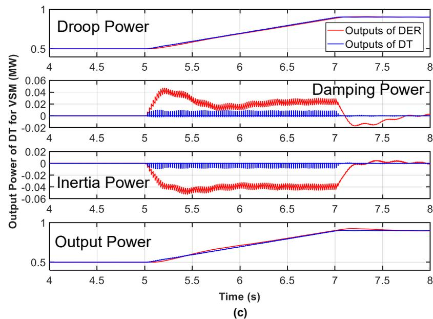
**Figure 12.** Time-step effect evaluation: (a) Time-step = 0.02 s; (b) Time-step = 0.002 s. (c) Time-step = 0.0002 s
