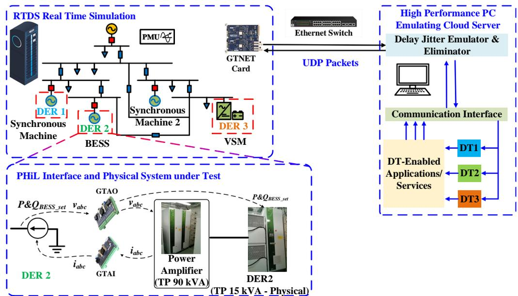
Figure 2. A representation of the DT-based real-time HiL platform.
