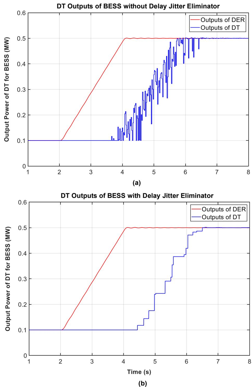
**Figure 10.** Effectiveness validation of jitter elimination on DT of BESS: (a) Comparison of original signal and signal with communication jitter (b) Comparison of original signal and signal after jitter elimination.
