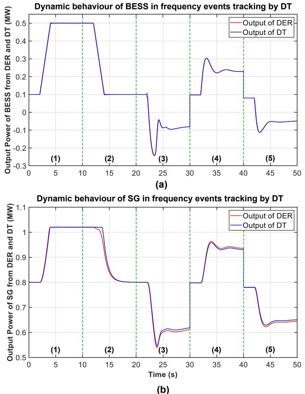
**Figure 8.** DTs of BESS and SG validation under five scenarios: (a) DT of BESS; (b) DT of VSM.
