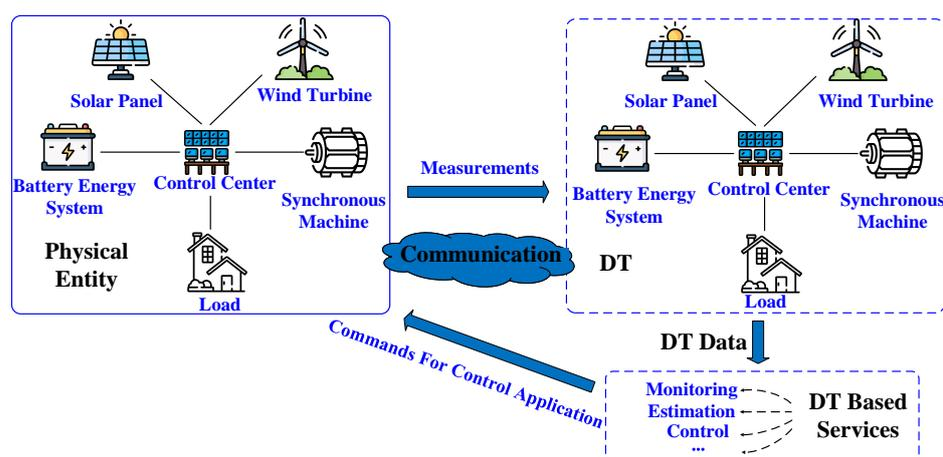
Figure 1. A typical five-dimension layout of a DT-based system.
