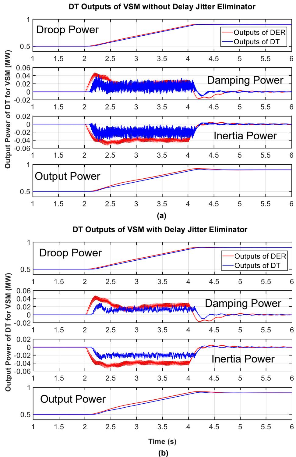
**Figure 11.** Effectiveness validation of jitter elimination on DT of VSM: (a) Comparison of original signal and signal with communication jitter (b) Comparison of original signal and signal after jitter elimination.
