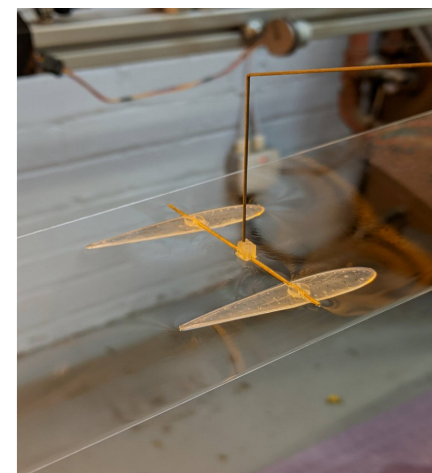
Fig 3 - Twin Rudder Arrangement in an Inclined Flowing Soap Film.
