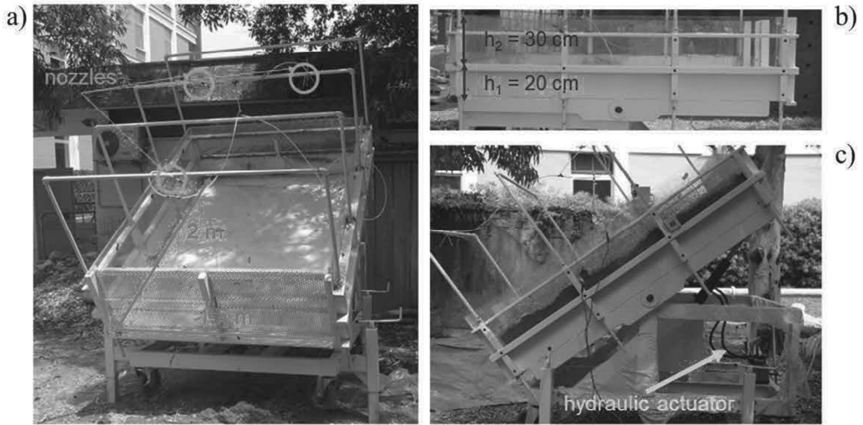
FIGURE 3: Slope physical model: (a) front view; (b) lateral view in horizontal position; (c) lateral view in tilted position
