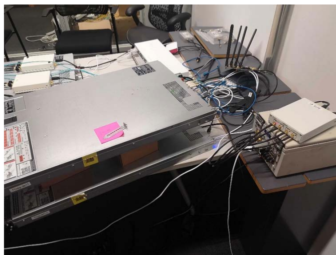
Figure 2-9 5G CBRS testbed in the lab with B210 RU
