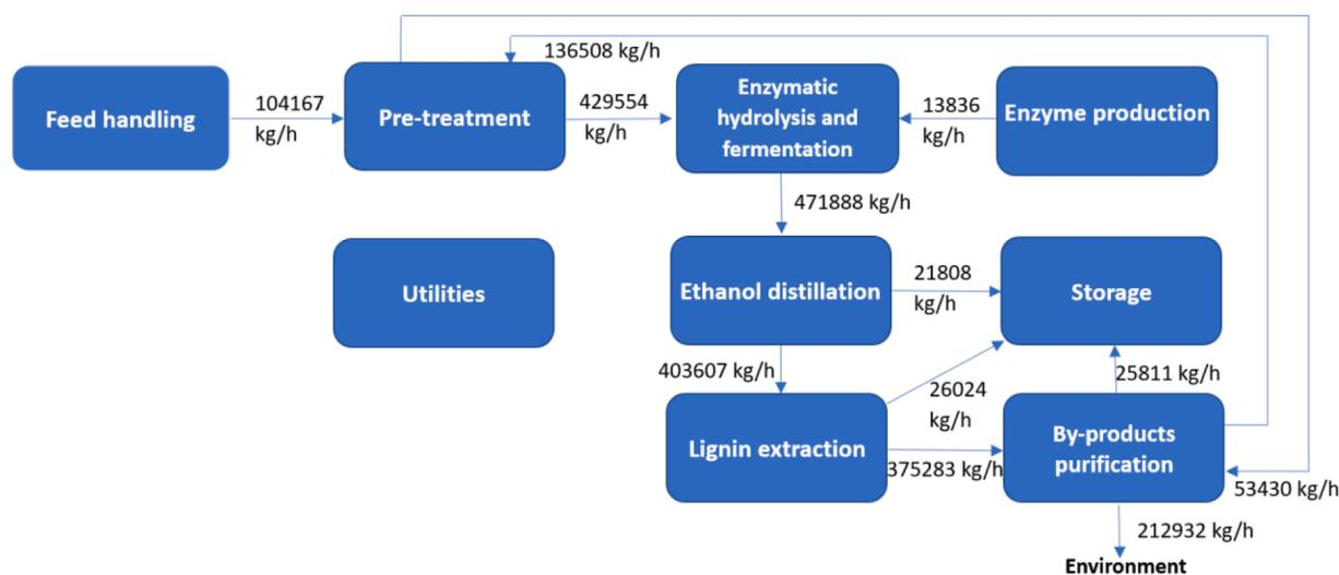
Fig. 4. The stream flow of zero waste ethanol biorefinery process.
