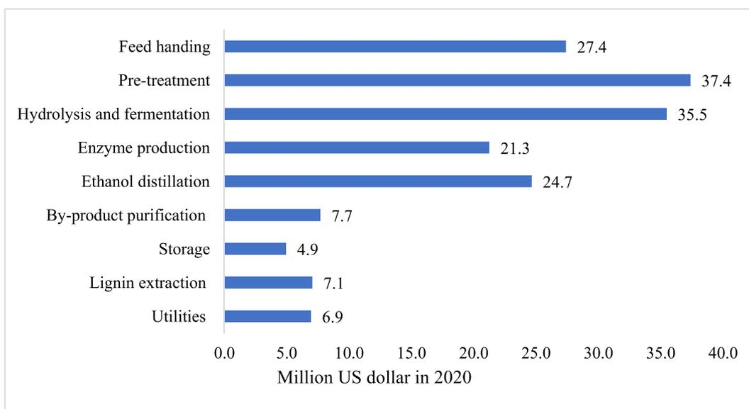
**Fig. 5.** Zero waste biorefinery plant capital cost breakdown by sub-processes.
