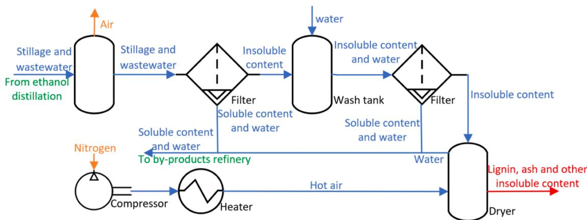
Fig. 2. Lignin extraction flowsheet in concept process diagram.
