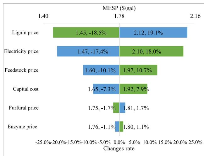
Fig. 7. The impact of parameters on MESP sensitivity.
