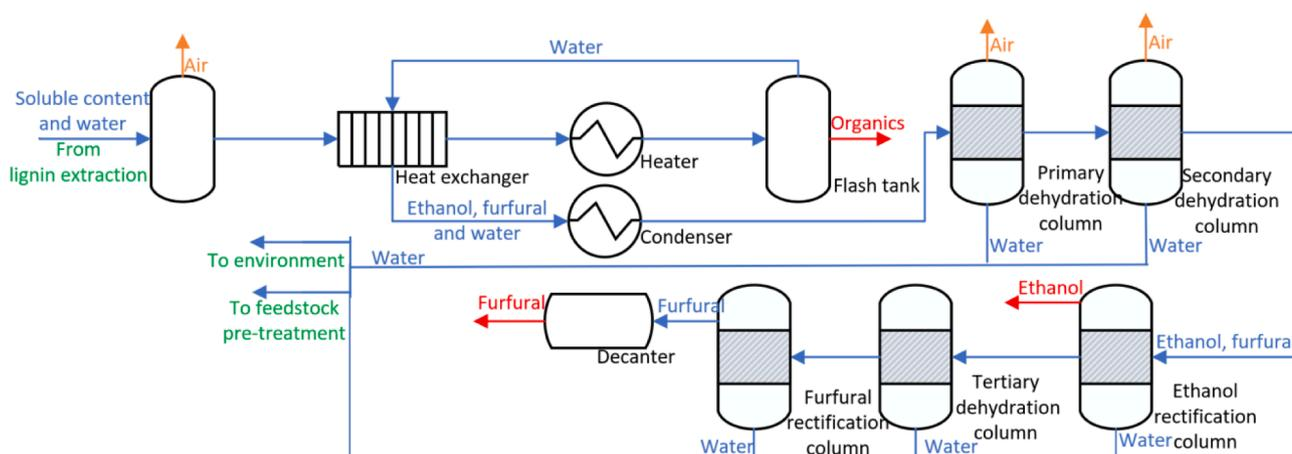
Fig. 3. Wastewater multistage purification process in concept process diagram.
