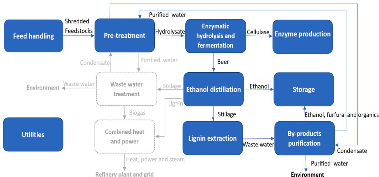
Fig. 1. Simplified flowsheet of zero waste and traditional (grey, [20]) ethanol biorefinery process.
