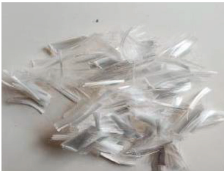
FIGURE 2: Modified polypropylene fiber.
