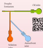
Droplets of supersaturated solution are formed at the Y-junction design element before being transported to a storage matrix where they can be observed for crystal nucleation. Droplets are of 0.5 nL volume.
