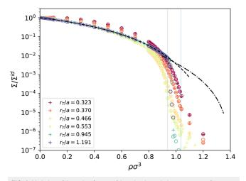
**FIG. 8.** Variation of the ratio of accessible tether bound phase space surface area with density at different fixed value of the tether length  $r_T/a$ . The pluses denote values calculated using  $\Delta S_T^{(\sigma)}$ , and the circles denote values calculated using  $\Delta S_T^{(r_T)}$ . The black dashed line is the residual free energy of the untethered hard sphere FCC solid.<sup>14</sup>
