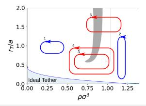
**FIG. 9.** Schematic diagram of states for tethered a hard sphere system. The blue shaded region denotes conditions where the system behaves as an ideal tether model. The dark gray shaded region is a qualitative depiction of the region where the entropy estimated to be non-analytic.
