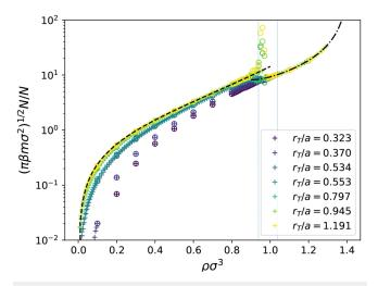
**FIG. 5.** The particle–particle collision rates of the tethered hard sphere model. The crosses are the data from the MD simulations, and the open circles are from the density derivatives of  $\Delta S_7^{(r_7)}/k_B$ , the entropy calculated via integration of the tether event rate. The black dashed line is the Carnahan–Starling<sup>13</sup> equation of state, while the black dashed–dotted line is the equation of state developed by Pieprzyk *et al.*<sup>14</sup> for the solid FCC phase.
