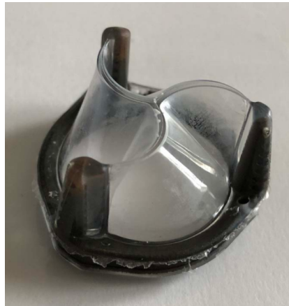
Figure 1: The Wheatley Valve. The height is 13 mm and the outer diameter is 25 mm; the inner orifice diameter is 23mm. A typical leaflet thickness is 150 microns.
