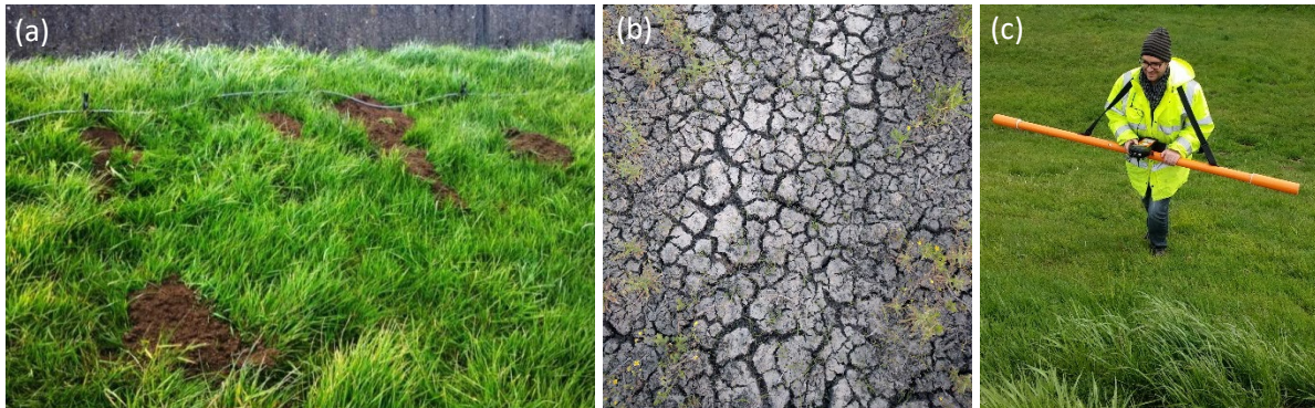
Figure 5: (a) Visual signs of excavated soil indicating the presence of mole-hills located in the upper part of the downstream shoulder of the embankment, (b) clay fissuring detected on the north-east side of the dam (c) EM survey carried out over the surface of Holl dam.
