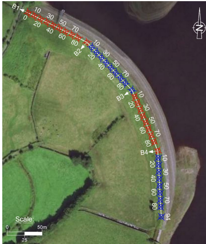
Figure 15: Non-intrusive ERT arrays (B1, B2, B3 and B4) 96m long with 2m electrode spacing covering the crest length of Barcraigs dam.
