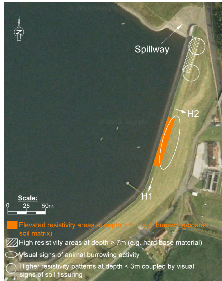
Figure 9: Visual correlation of findings derived from visual inspection and geophysical assessment of Holl reservoir dam.
