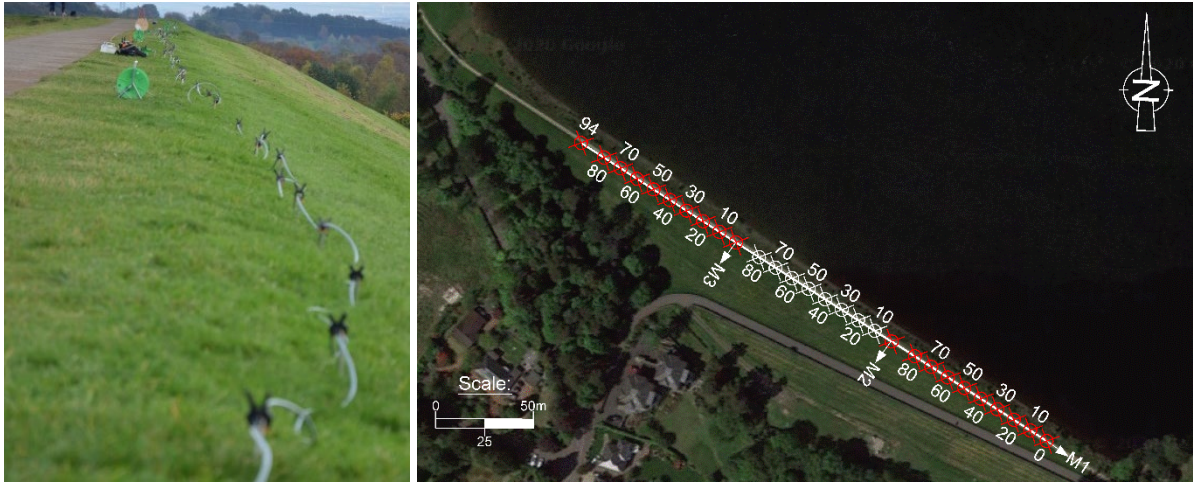
Figure 10: (a) Non-intrusive geophysical investigation with ERT arrays installed on the crest of Mugdock reservoir dam, (b) ERT arrays (M1, M2 and M3) with length of 96 m and electrode spacing intervals of 2 m covering part of the length of Mugdock dam.
