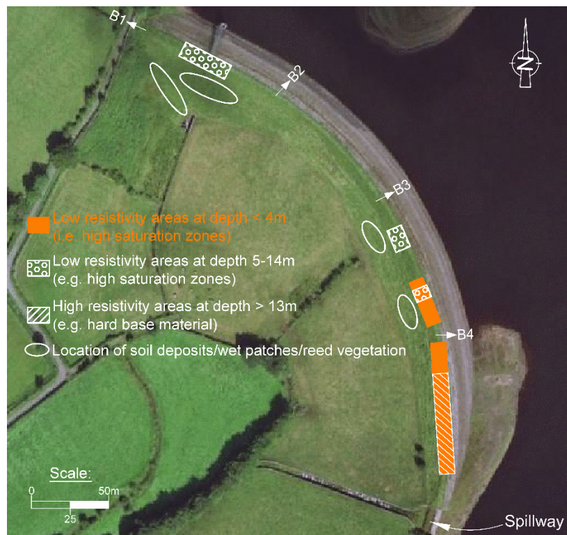
Figure 18: Visual correlation of findings derived from visual inspection and geophysical assessment of Barcraigs reservoir dam.
