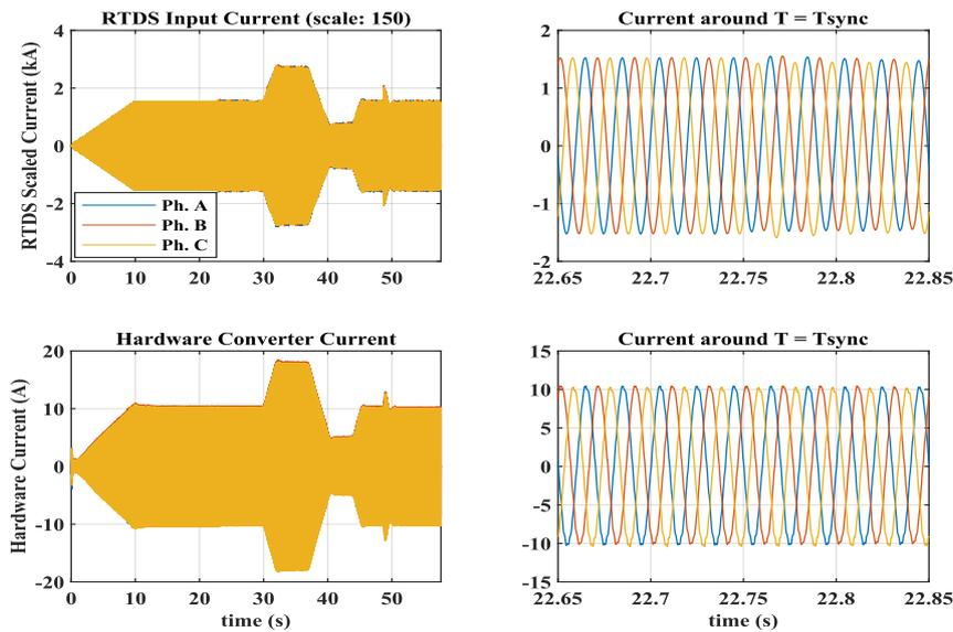
**Figure 6: RTDS vs. Hardware Input Current Measurements.**
