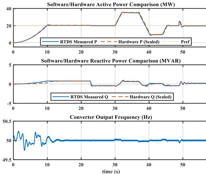
Figure 7: PHiL Active and Reactive Power Tracking Performance (Software vs. Hardware), and GFC frequency.
