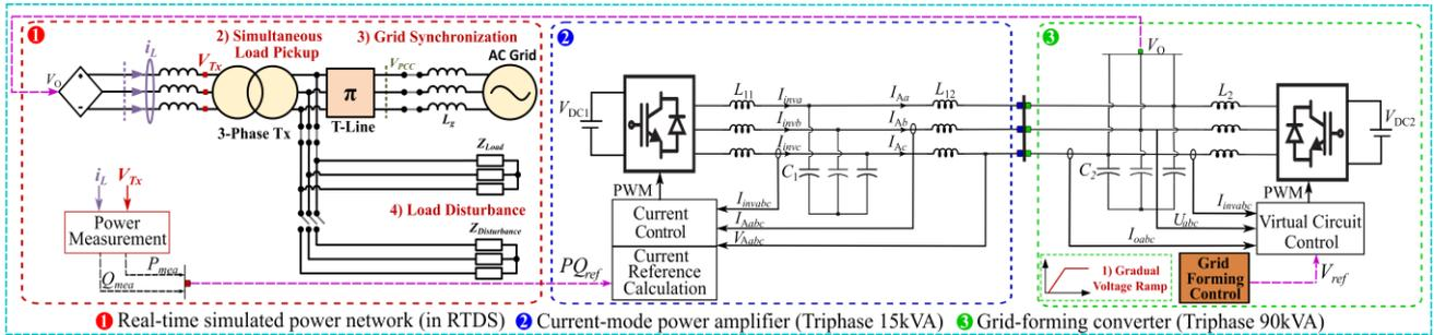
**Figure 3: Equivalent circuit diagram of the PHIL setups.**
