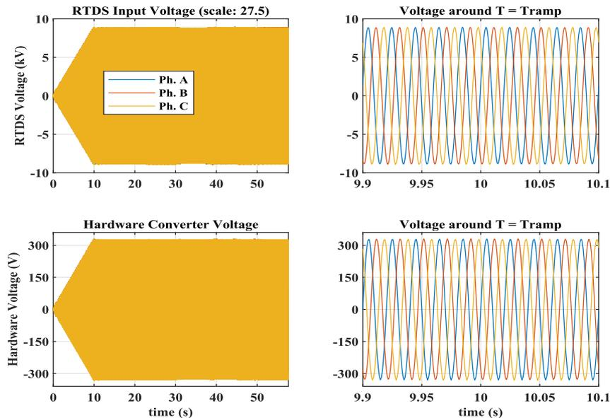
Figure 5: RTDS vs. Hardware Input Voltage Measurements.
