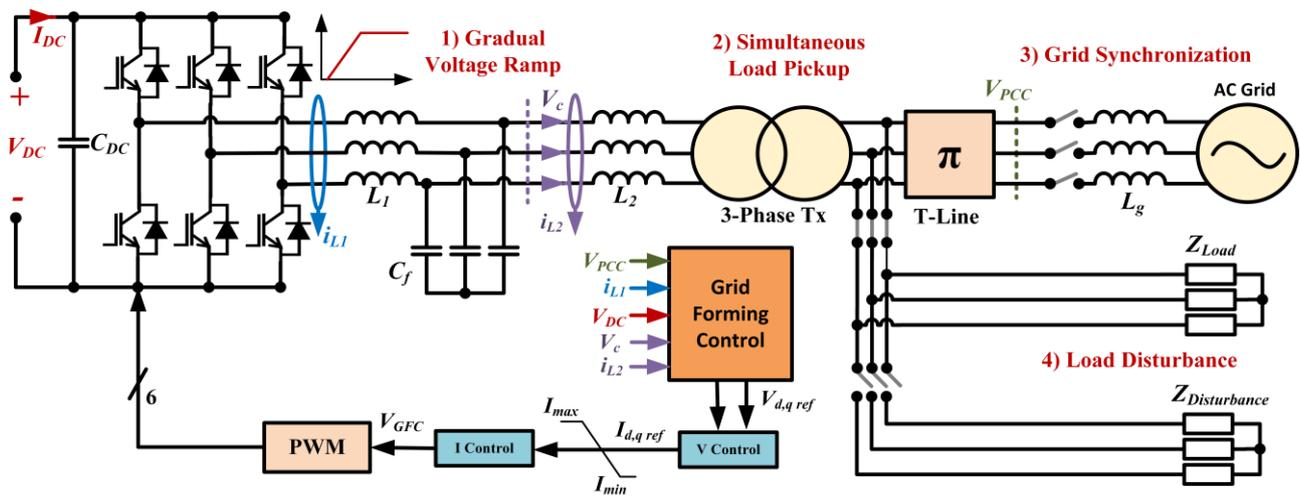
Figure 2: Test network block-diagram used for black-start experiments.
