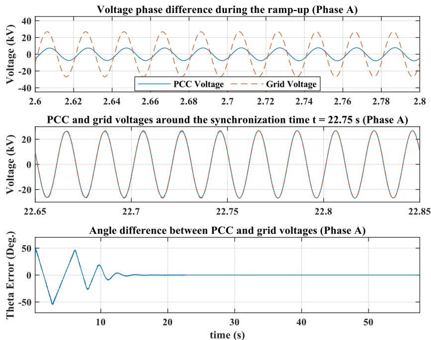
Figure 8: Synchronizing control impact in reducing the phase shift between PCC voltage and grid before synchronization.
