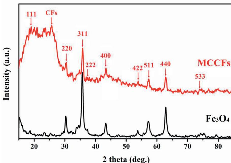
Fig. 1. Typical XRD patterns of as-synthesized nano- $\text{Fe}_3\text{O}_4$  powder and MCCFs.
