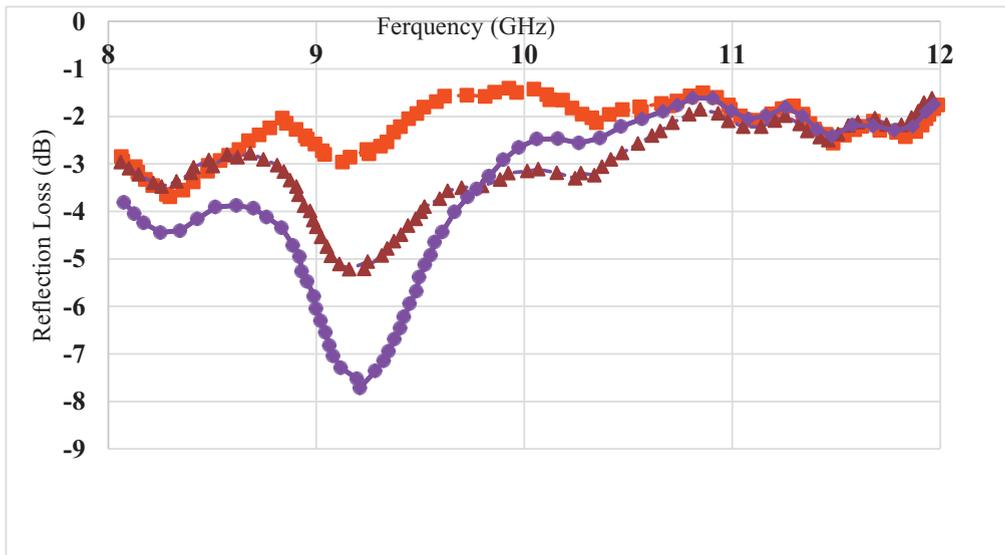
Fig. 6. Reflectivity curves of samples coated in (a) one; (b) two; (c) three steps.
