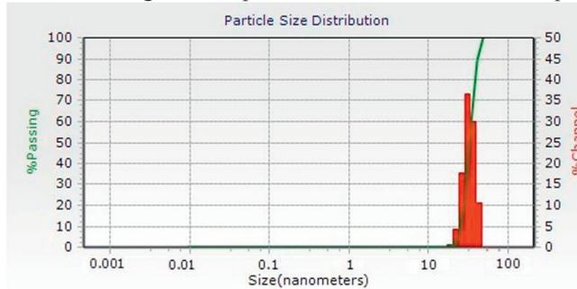
Fig. 3. Particle size distribution of  $\text{Fe}_3\text{O}_4$  particles as a function of volume of  $\text{Fe}_3\text{O}_4$  particles.
