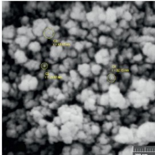
Fig. 2. FE-SEM image of the as-prepared  $\text{Fe}_3\text{O}_4$  nanoparticles.
