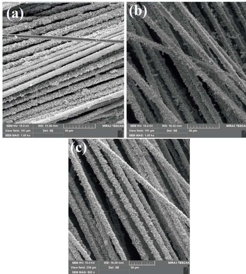
Fig. 4. FE-SEM images of MCCFs coated in (a) one step; (b) two steps; (c) three steps.
