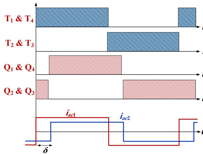
Fig. 2: Proposed LCC-DAB modulation principle.
