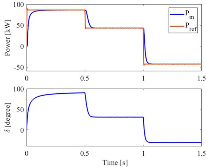
Fig. 8. Simulation results when varying the power transfer amount and direction.
