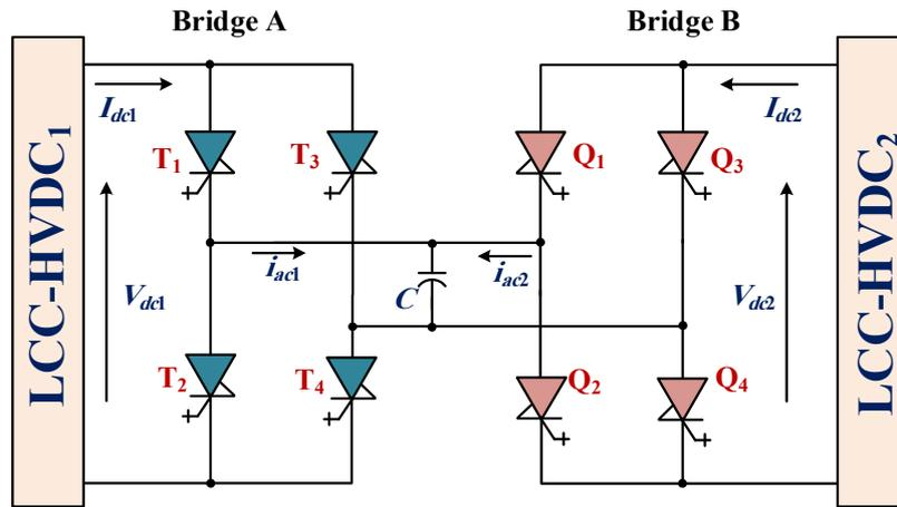
Fig. 1: Proposed dc-dc converter.
