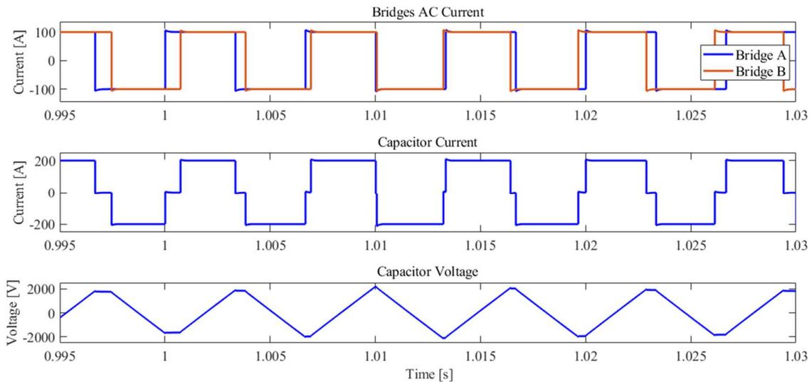
Fig. 9. Simulation results for the capacitor voltage and current during the power reversal period.
