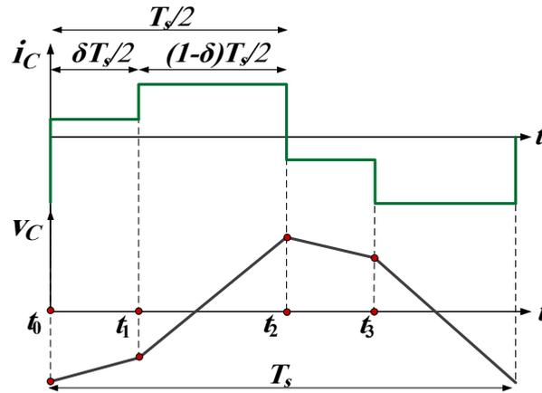
Fig. 5: Generic capacitor voltage waveform.
