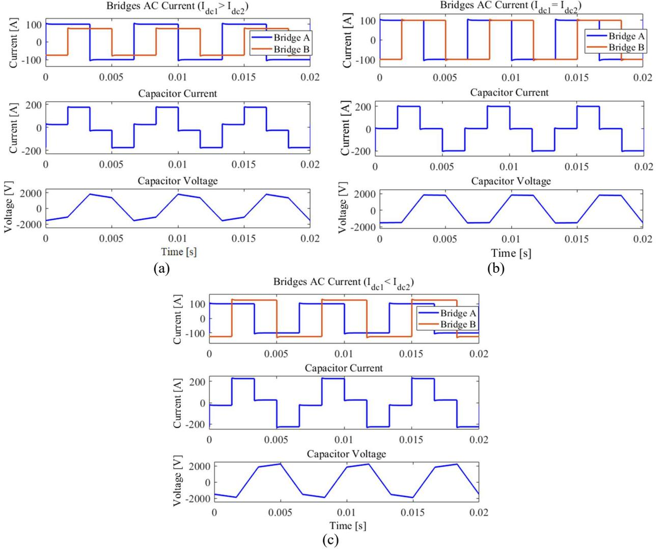
Fig. 7: Simulation results when varying the dc-link current levels. (a)  $I_{dc1} > I_{dc2}$ . (b)  $I_{dc1} = I_{dc2}$ . (c)  $I_{dc1} < I_{dc2}$ .
