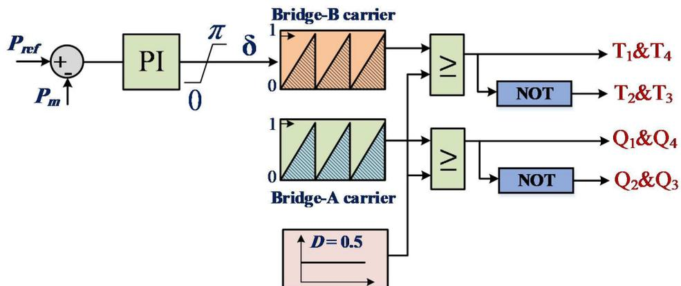
Fig. 4: LCC-DAB phase-shift control principle.
