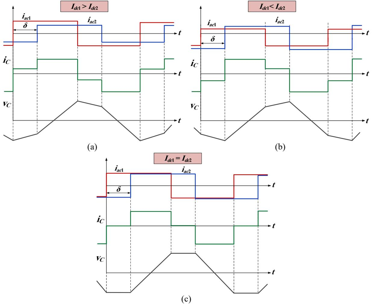
Fig. 6: Variation of capacitor voltage waveform based on the difference in dc-link currents.
