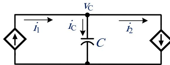
Fig. 3: Simplified LCC-DAB circuit.
