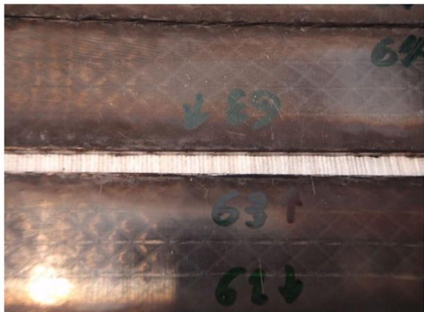
341  $\mu\text{m}$  for cuts using a 2.0 mm aperture and 345  $\mu\text{m}$  using 1.0 mm aperture. The double aperture nozzle works by generating a flow of high-pressure air directed downwards on the surface and less air is directed radially. This reduces the pressure that forces the top epoxy layer away from the laser radiation or gas flow during processing.
