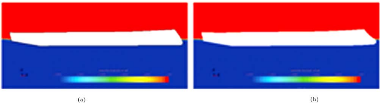
Figure 18. Free surface elevation of the initial (a) and the optimized (b) hull at speed 16 knot.
