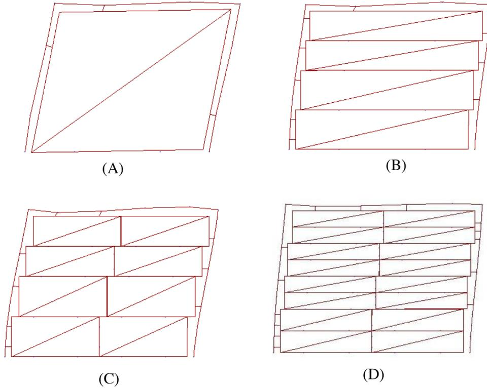
FIGURE 11 Deformed shapes of (A) TIF, (B) IFSJ (4 × 1 mesh), (C) IFSJ (4 × 2 mesh), (D) IFSJ (8 × 2 mesh)
