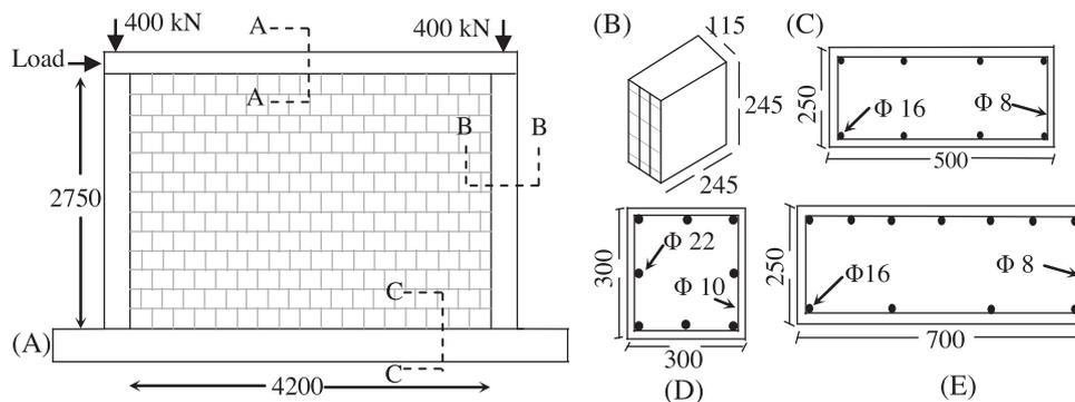
**FIGURE 5** Geometric details (dimensions in mm) of (A) the tested infilled frame (B) the perforated clay block units, (C) top beam (section A-A), (D) column (section B-B), and (E) top beam (section C-C)
