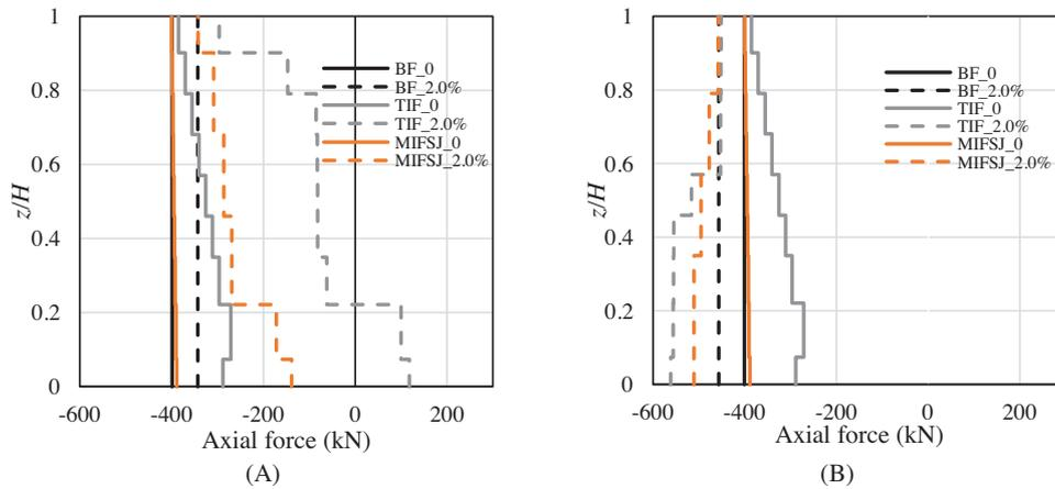
FIGURE 12 Comparisons of axial forces in BF, TIF (4 × 1 mesh) and IFSJ (4 × 1 mesh) for (A) windward column (B) leeward column
