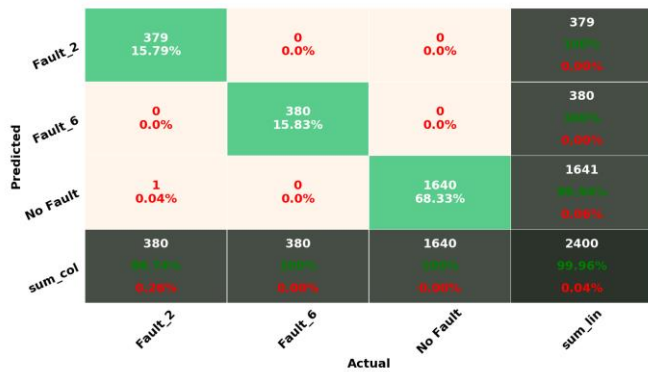
Figure 13: Confusion matrix for knowledge extracted using the manual approach. Five samples per datastream manual technique properly classified all defects.
