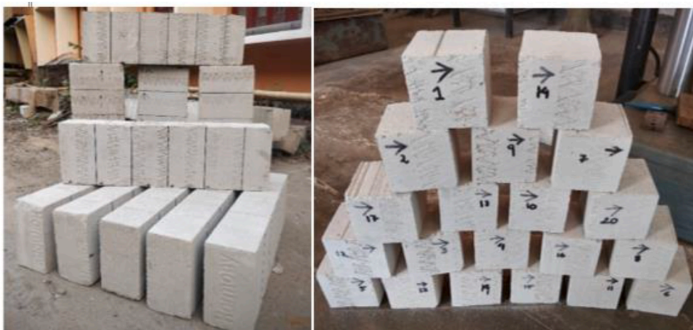
Fig. 2. AAC blocks (a) as procured and (b) cube specimens used for the experiments.
