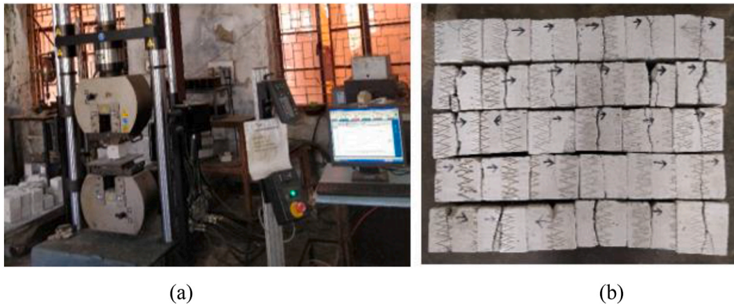
Fig. 7. (a) test setup for the split tensile test (b) AAC samples after the split tensile test.
