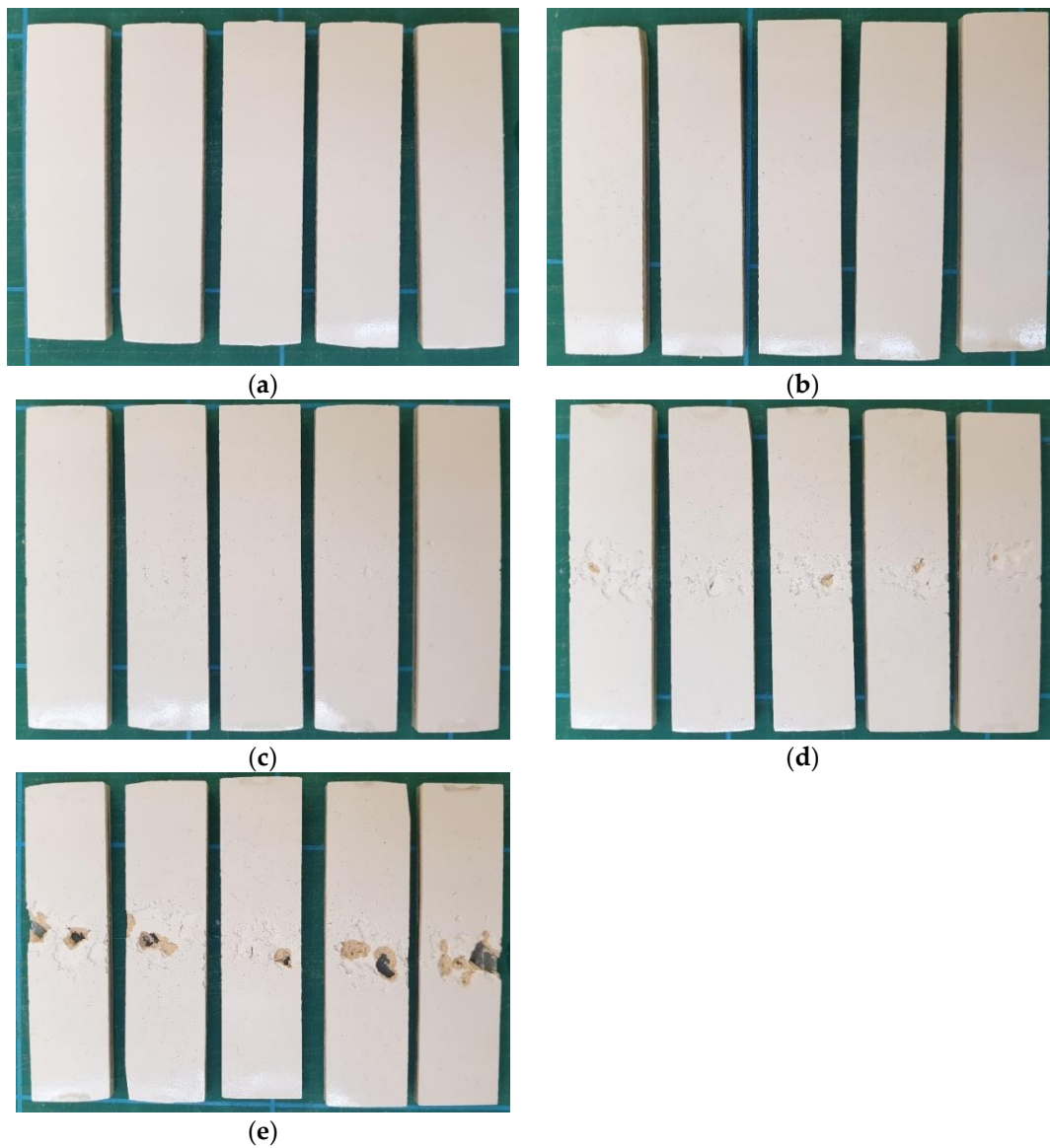
Figure 8. (a) Samples with coating C at stage 1; (b) samples with coating C at stage 2; (c) samples with coating C at stage 3; (d) samples with coating C at stage 4; (e) samples with coating C at stage 5.
