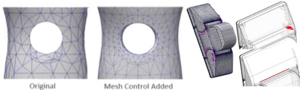
Figure 4. (a) interdental cleaning product mesh; (b) multi-part assembly
