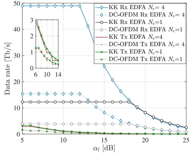
Fig. 3: The achievable data rate with a total power less than the eye-safety limit and the BER less than the FEC threshold using 16-QAM modulation format. Values for DC-OFDM and KK systems are presented for various link losses, fiber cores, and optical amplification at the transmitter or receiver sides.
