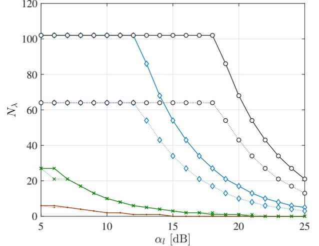
Fig. 4: The maximum number of wavelength channels,  $N_\lambda$ , with a total power less than the eye-safety limit and the BER less than the FEC threshold using 16-QAM modulation format. Values for DC-OFDM and KK systems are presented for various link losses, fiber cores, and optical amplification at the transmitter or receiver sides.
