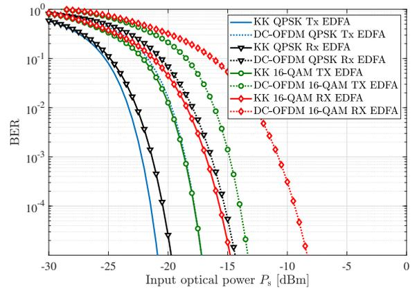
Fig. 2: The BER values for IM/DD and KK systems for different values of input signal power, modulation format, and optical amplification at the transmitter or receiver sides. Quadrature Phase Shift Keying (QPSK).
