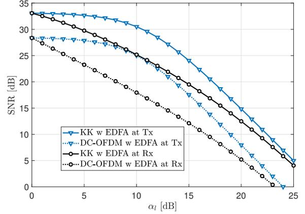
Fig. 1: The SNR values for IM/DD and KK systems for different values of link loss and optical amplification at the transmitter (Tx) or receiver (Rx) sides.
