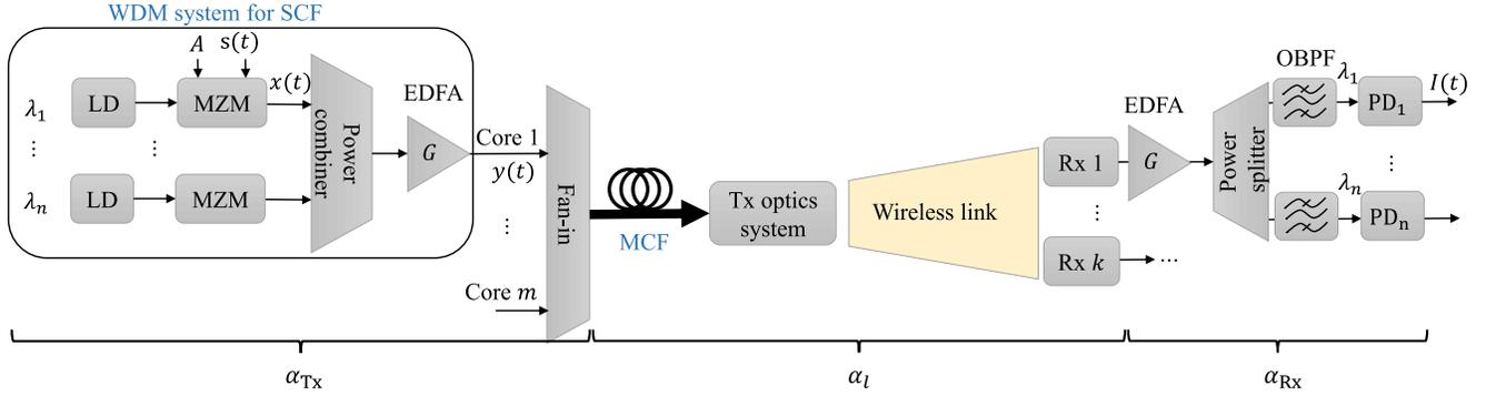
Fig. 1: The block diagram of the system. single core fiber (SCF), laser diode (LD), Mach-Zehnder modulator (MZM), multi-core fiber (MCF), Erbium-doped fiber amplifier (EDFA), receiver (Rx), optical bandpass filter (OBPF), photodiode (PD).
