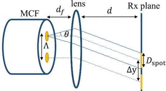
Fig. 2: The ray diagram of the optics system.
