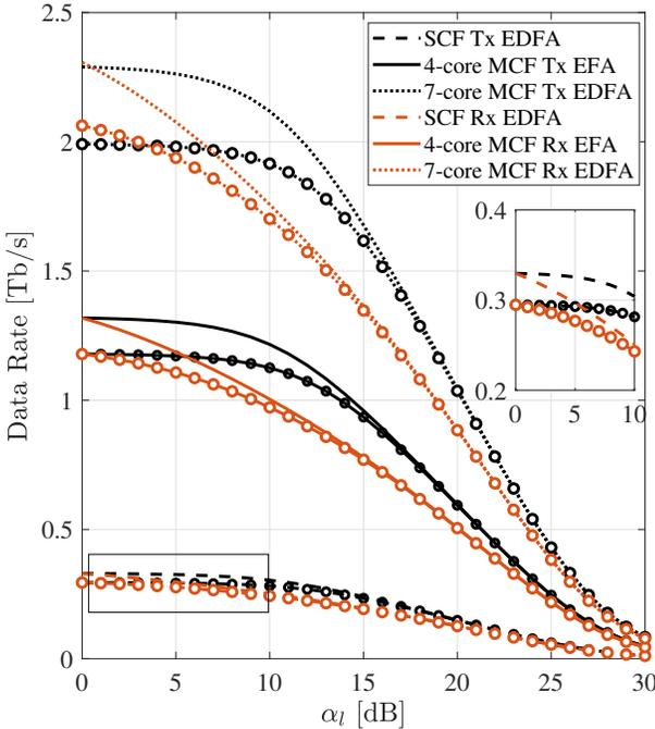
Fig. 5: Achievable data rates for SCF, 4-core, and 7-core MCFs per wavelength. Marked lines are for  $L = 10$  km. The inset plot shows the magnified SCF curves. When  $L$  changes from 1 to 10 km,  $\alpha_l$  also increases by 1.8 dB.
