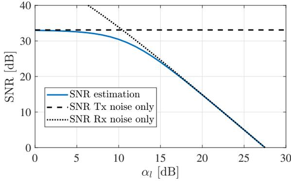
Fig. 4: The comparison of SNR estimation with the SNRs when only either Tx or Rx noises are considered for a 4-core MCF at  $P = -10$  dBm and
