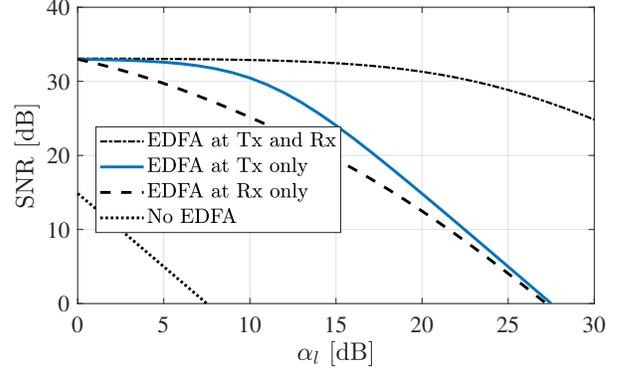
Fig. 3: SNR estimations versus link loss for different amplification strategies for a 4-core MCF at  $P_s = -10$  dBm and  $\text{CSPR} = 10$  dB.
