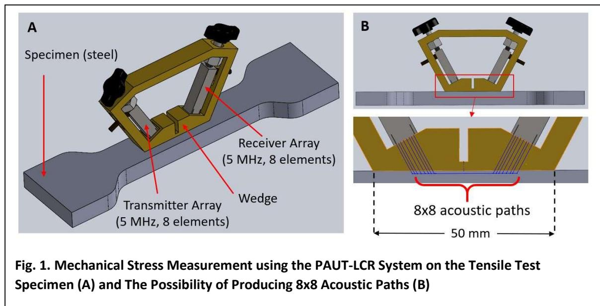
**Fig. 1. Mechanical Stress Measurement using the PAUT-LCR System on the Tensile Test Specimen (A) and The Possibility of Producing 8x8 Acoustic Paths (B)**
