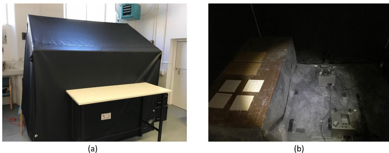
Figure 1 - Cyanoacrylate Fuming Tent: (a) exterior and (b) interior set-up example
