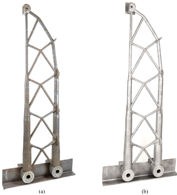
FIGURE 18. Cantilever truss (a) before and (b) after sandblasting.
