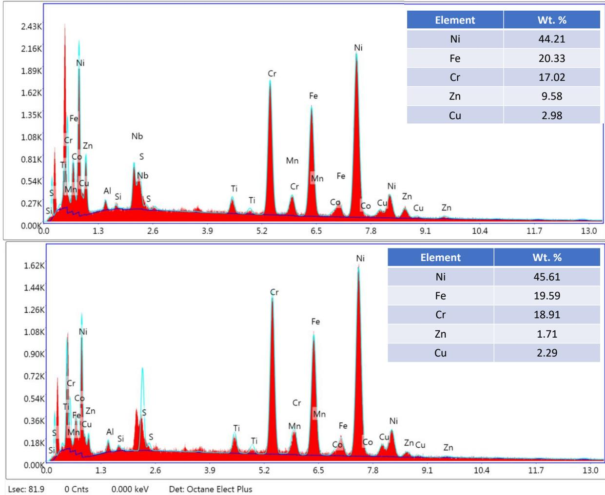
**Fig. 8** EDS analysis of surface machined with hard zinc coated brass wire under
