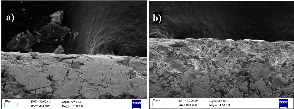
**Fig. 10** SEM images of hard zinc coated brass wire surface at discharge energy mode (a) C1 (b) C5
