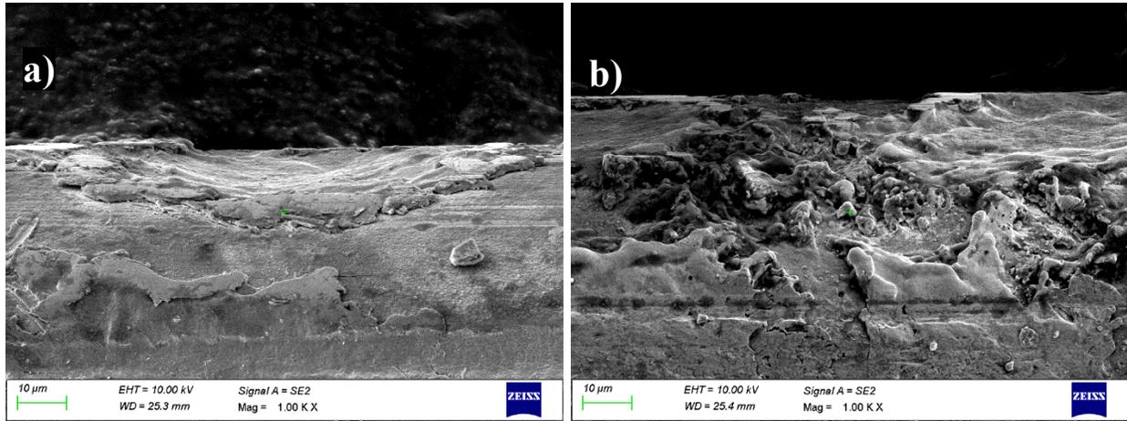
**Fig. 12** SEM images of hard uncoated brass wire surface at discharge energy mode
