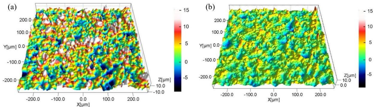
**Fig. 4.** 3D surface morphology of Inconel 718 machined with hard zinc coated brass electrode at
