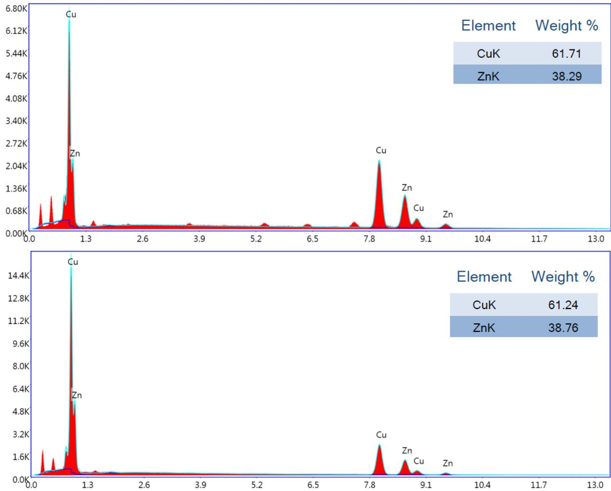
**Fig. 13** EDS images of hard uncoated brass wire surface at discharge energy mode
