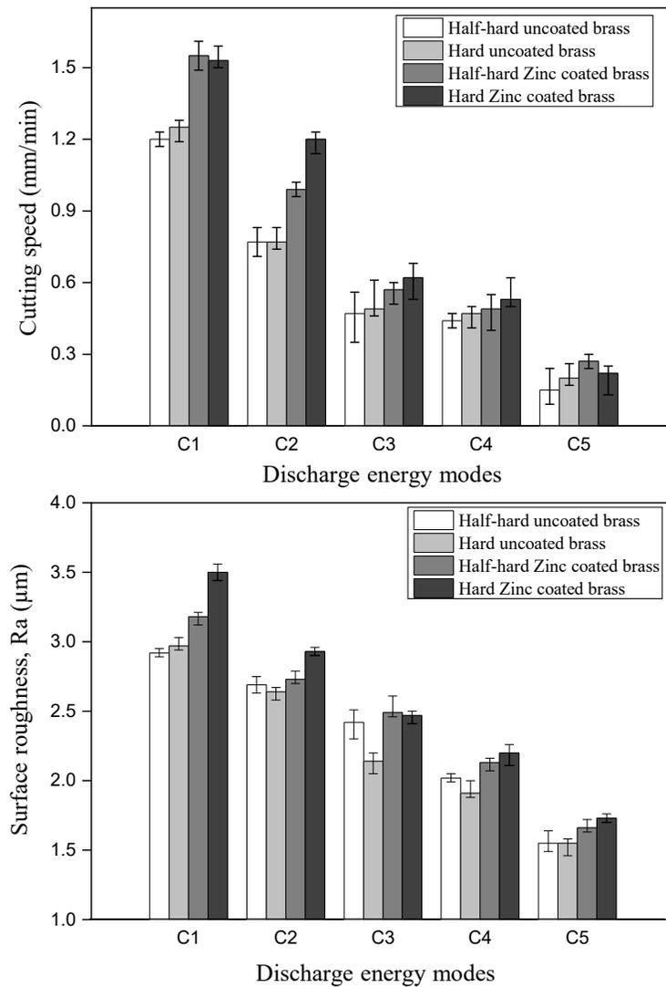
**Fig. 3.** Effect of wire material and discharge energy on (a) cutting speed (b) surface roughness ( $R_a$ )
