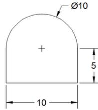
**Fig. 1.** Profile of the part machined (All dimensions in mm)
