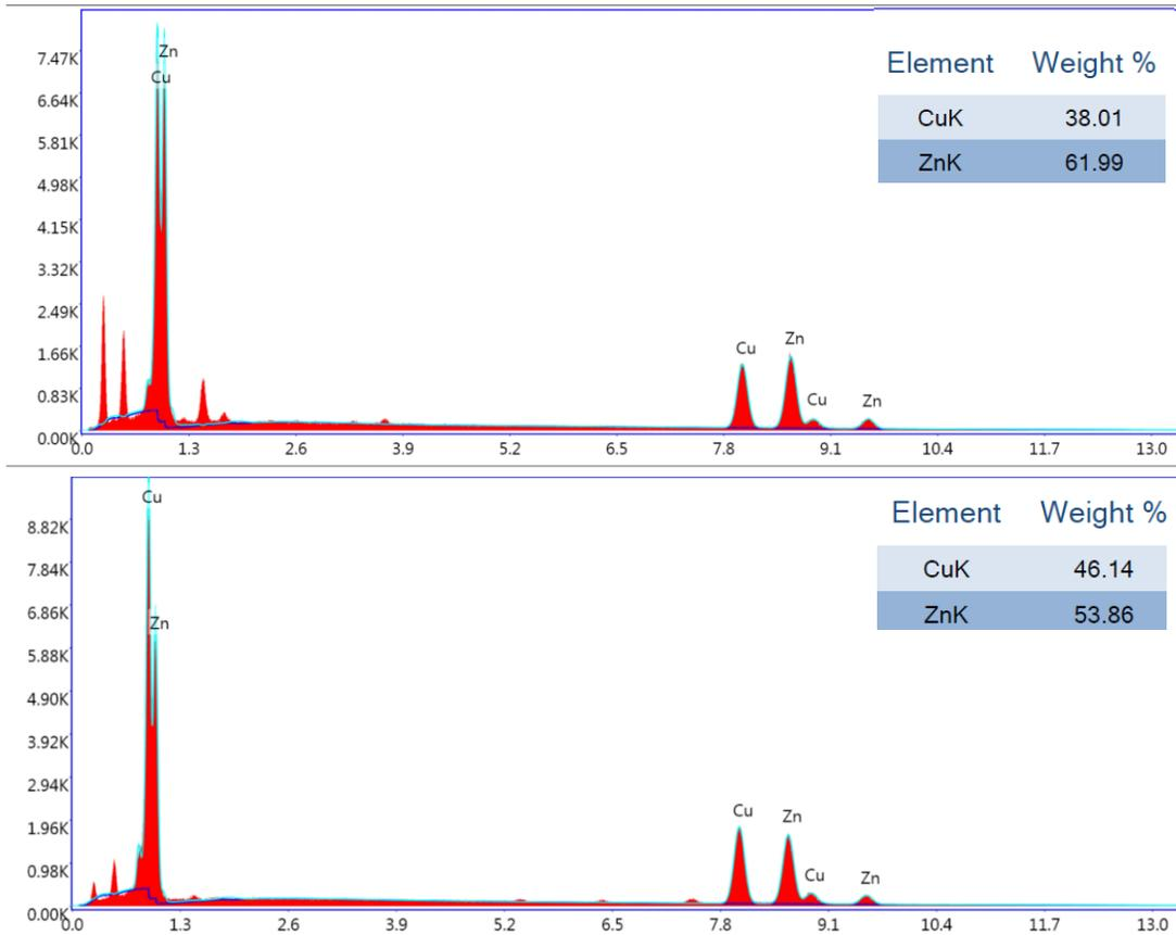
**Fig. 11** EDS images of hard zinc coated brass wire surface at discharge energy mode (a) C1 (b) C5
