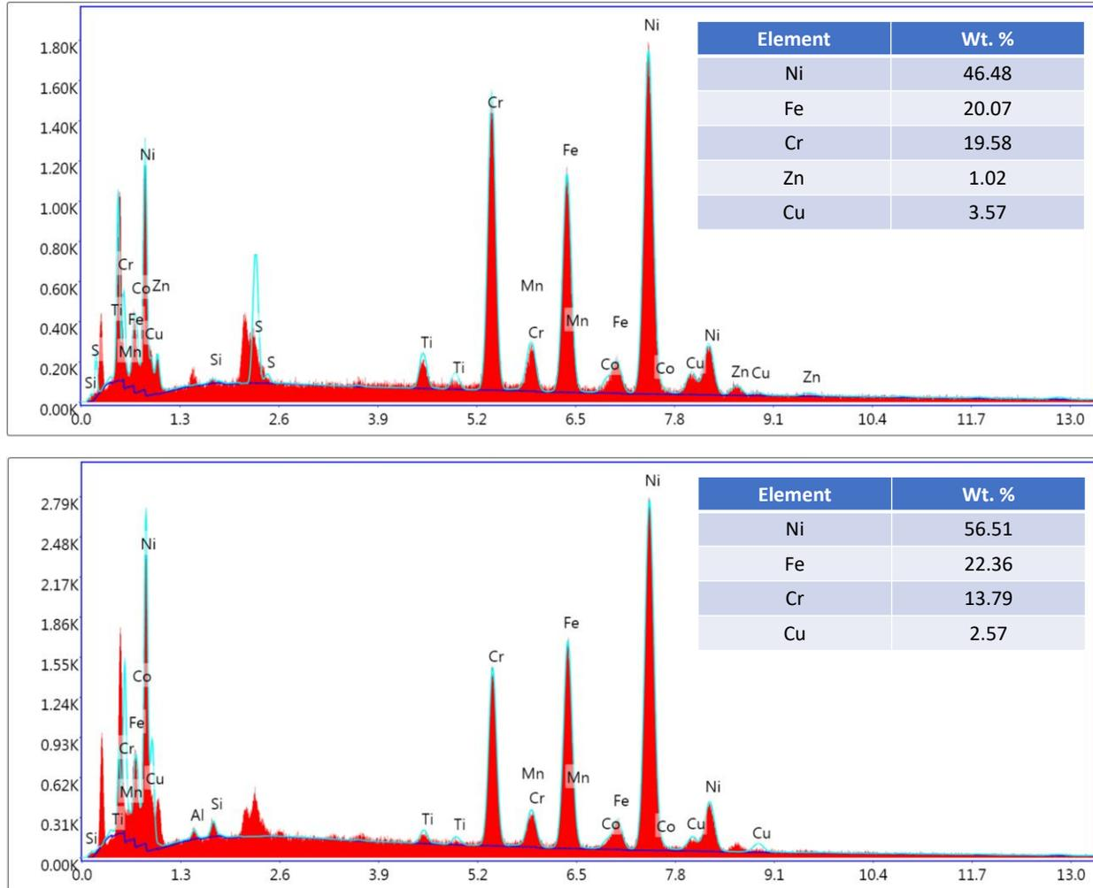
**Fig. 9** EDS analysis of surface machined with hard uncoated brass wire under
