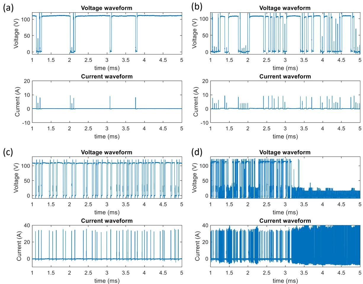
**Fig. 14.** Comparison of pulse discharge cycles at various discharge energy levels
