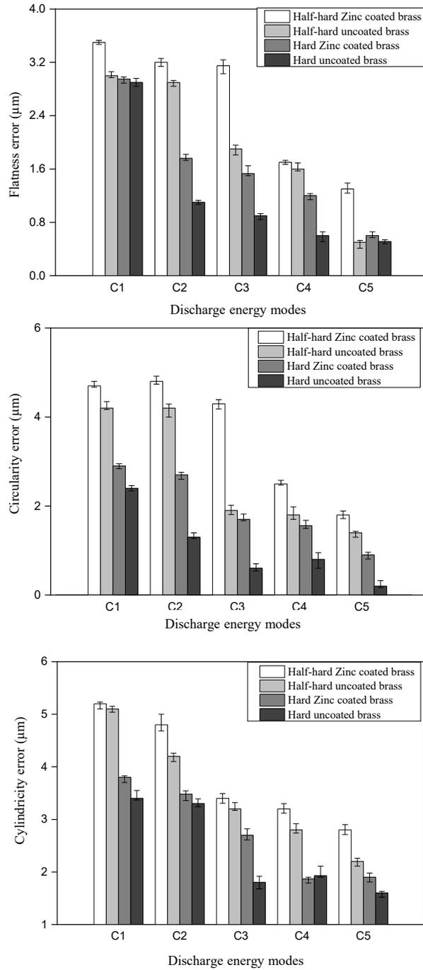
**Fig. 5.** Effect of wire material and discharge energy on geometrical accuracies
