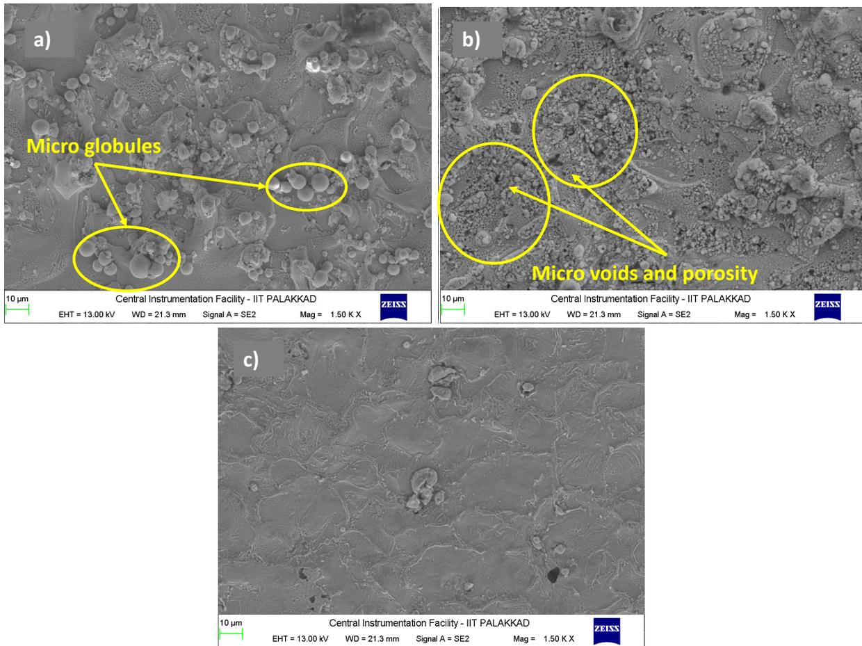
**Fig. 6.** SEM images of machined surface at discharge energy mode
