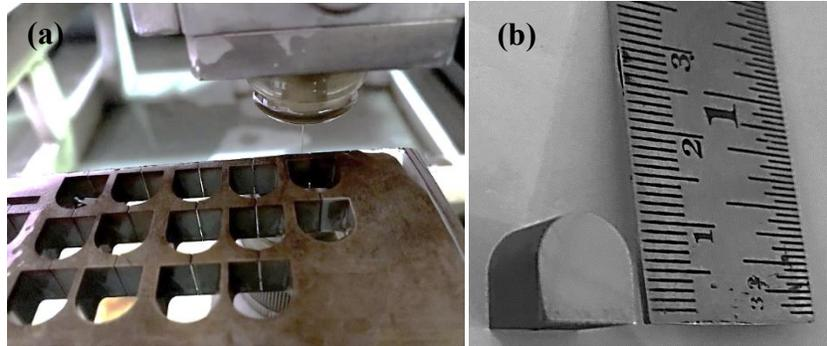
**Fig. 2.** (a) Multiple slots after a few profiles were cut; (b) A single cut specimen with dimensions
