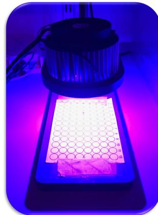
**Fig. 1.** 405-nm LED array for exposure of bacterial samples to 5 and 50 mWcm<sup>-2</sup> irradiances.
