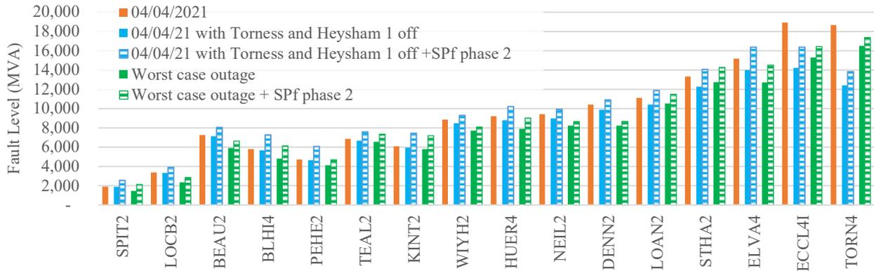
Figure 4: Fault level contribution from Stability Pathfinder Phase 2 (assumed solutions)
