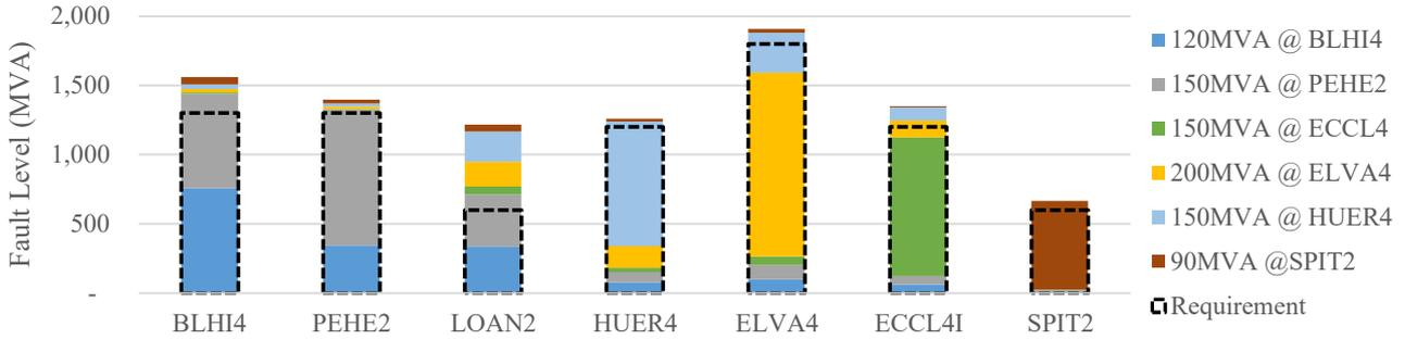
Figure 3: Modelled solutions to stability pathfinder and their fault level contribution at each area of requirement.
