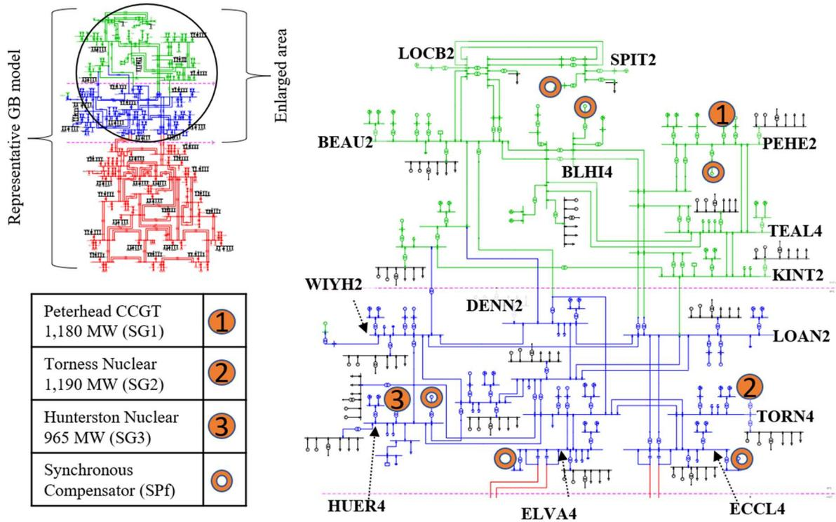
Figure 1: Representative GB power system model - including enlarged Scottish area showing location of main SGs and assumed locations of synchronous compensation from the NG ESO SPf Phase 2 tender
