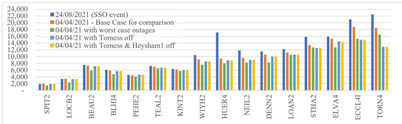
Figure 2: Fault levels for base-case, SSO case, and the effects of equipment outages and SGs being offline
