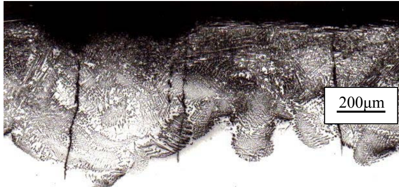
18.4 Laser induced cracks through the entire depth of the melt pool arrested at the HAZ. (Mridha and Baker 1991)
